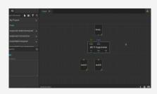
Play the video on this slide to demonstrate Task 3 (p34-35), which uses a *tweak* node to initiate readings from the temperature and humidity sensor, and *watch* nodes to view the results.
